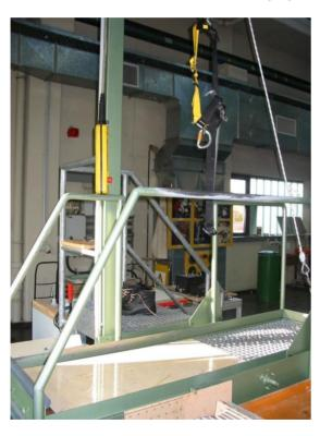
"Walking" on a slippery test floor until it becomes unsafe.
